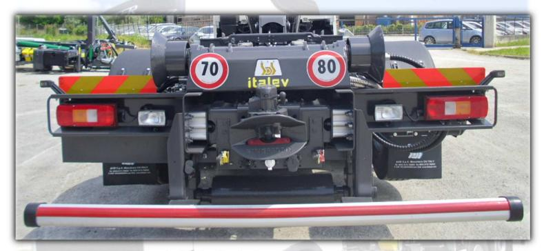
The rear lights block is bolted. The lights are in upper and protected position.
