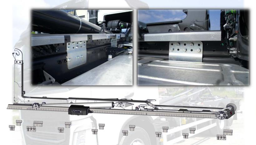
The pierced longitudinal hooklift beams allow the bolting instead of welding of the plates; thus resulting a perfect coupling going with mounting time reduction.
