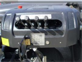
The control system Bobeasy is made of: wire control in the cab, receiver on the ground, levers for emergency, and radio control in option.
