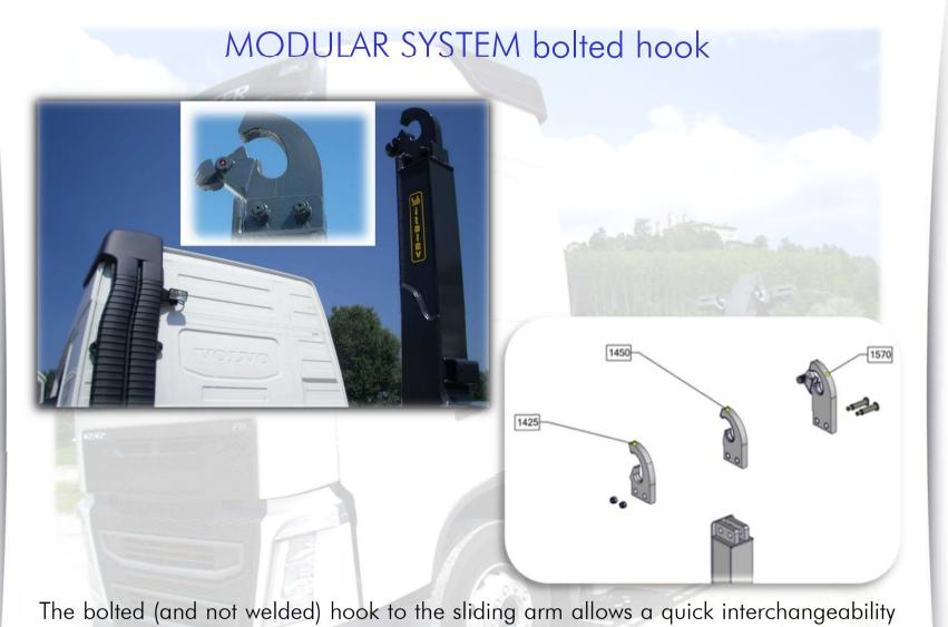
The bolted (and not welded) hook to the sliding arm allows a quick interchangeabilit in case of assistance or different hook heights needed.
