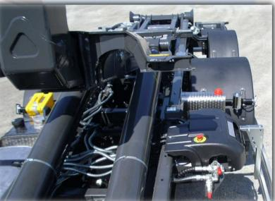
The modular system offers the possibility of bolting mudguards' brackets, cyclists' protection and storage boxes, further to the mounting of flexible hoses protections.
