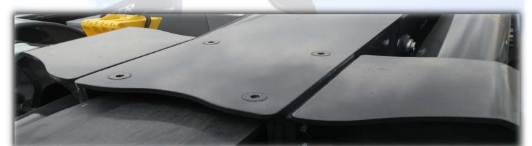
Upper, lower and lateral translation surface of the telescopic arm to grant a smoother movement during loading and container translation from/to the trailer.
