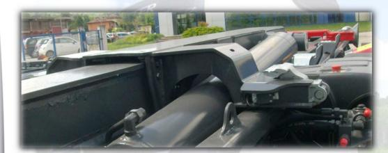
The front arms bolted to the central body sustain the container and together with the integrated locking they make transport and container tipping safe.
