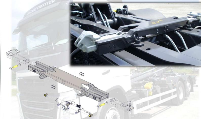
Standard hydraulic container locking with external forks. Possibility to reverse to internal fork locking according to DIN 30722 norm.
